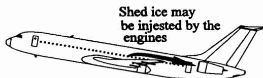
Fig. 12.3 Possible FOD by shed ice.
