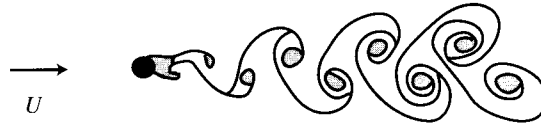
Figure 16.4 Schematic of the vortex street wake that forms downstream of a circular cylinder. The vortices are indicated by gray patches and the vortex sheets are black lines. Based on flow visualization of S. Taneda, as shown in Van Dyke (1982).
