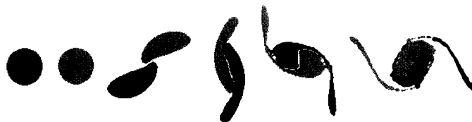
Figure 11.4 Merger of a pair of corotating vortices of equal strength, computed using the discrete-vortex method with adaptive amplitude fitting. The vortices initially have uniform vorticity with d/a = 3 . The vorticity field is plotted as a black or gray region, indicating vorticity originating from the left- or right-hand vortex, respectively, over five equal time increments.
