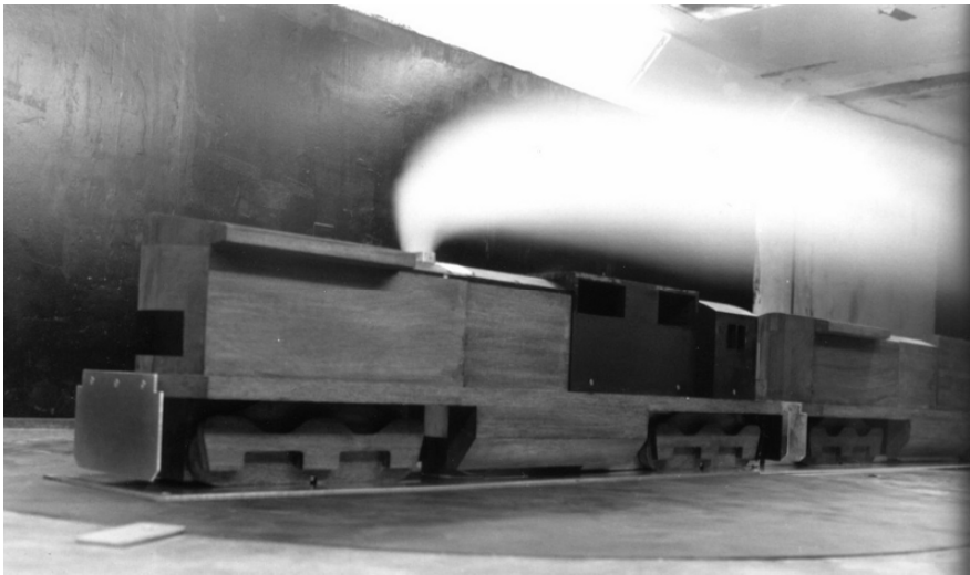
Fig. 16 Diesel Exhaust Plume Behavior, 1/15-Scale Wind Tunnel Test, Yaw Angle = 10^\circ , Long Hood Forward, with Auxiliary Blower in Operation.
