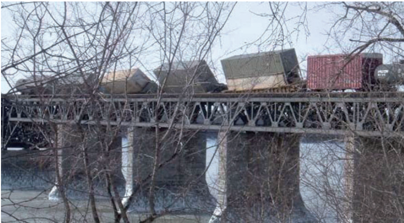
Fig. 8 Freight Train Derailment: 18 February 2006, Montreal Quebec, Kahnawake Bridge, 67 mile/hour crosswinds.
