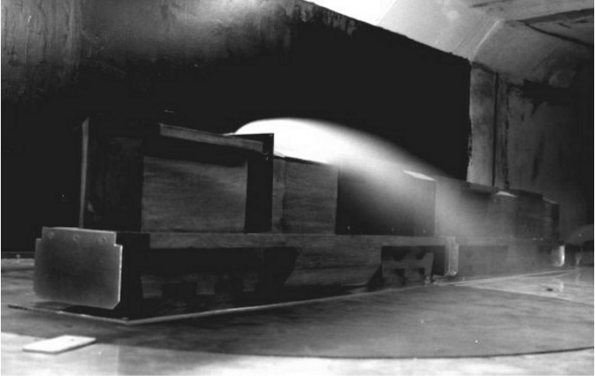
Fig. 15 Diesel Exhaust Plume Behavior: 1/15-Scale Wind Tunnel Test, Yaw Angle = 10^\circ , Long Hood Forward, Baseline Exhaust System
