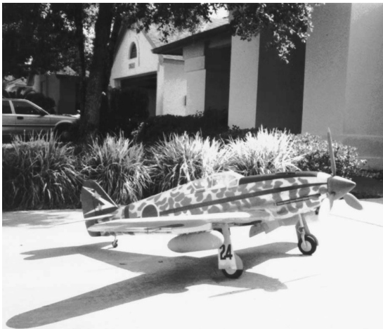
FIGURE 1.20 Model BF109 WWII German fighter plane using glass/epoxy-molded fuselage and wing spars of graphite/epoxy. (Photo courtesy of Russell A. Lepré, Tampa, FL.)
