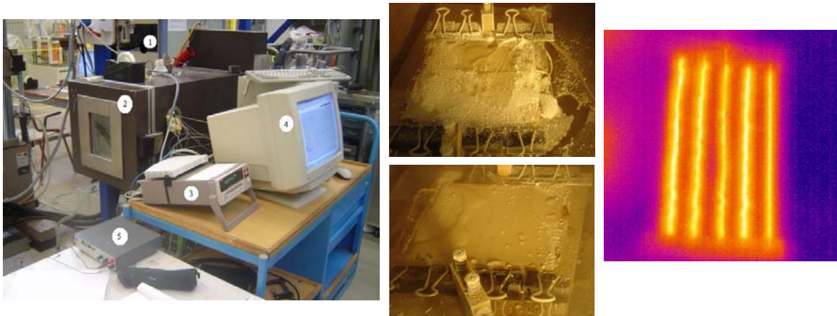
Figure 2. Climate chamber setup (left), panel with ice at -50^{\circ}\text{C} (top center), de-iced panel at -50^{\circ}\text{C} (bottom center), and infrared image of the HEL (right).
