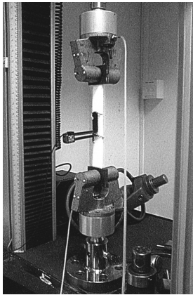
Figure 6: Tensile testing of headliner components
