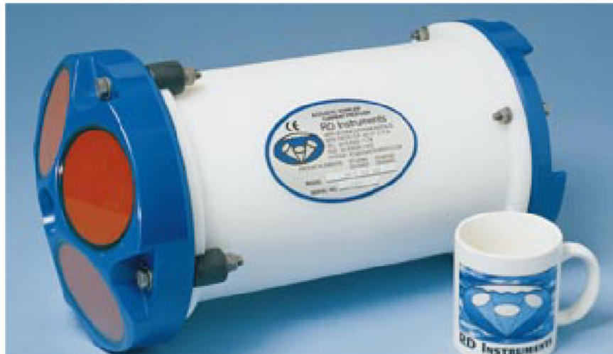
Figure 17- Workhorse Sentinel ADCP
