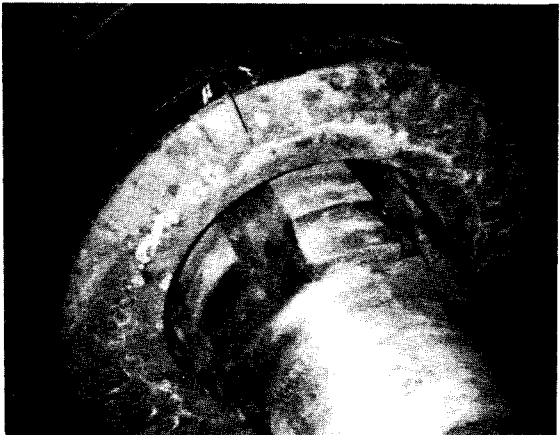
Fig. 4-30. Rotor with Broken Rotor Bar.
