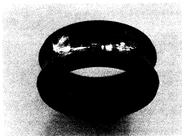
Fig. 5-40. Inner Race of Bearing with Acid Etching.
