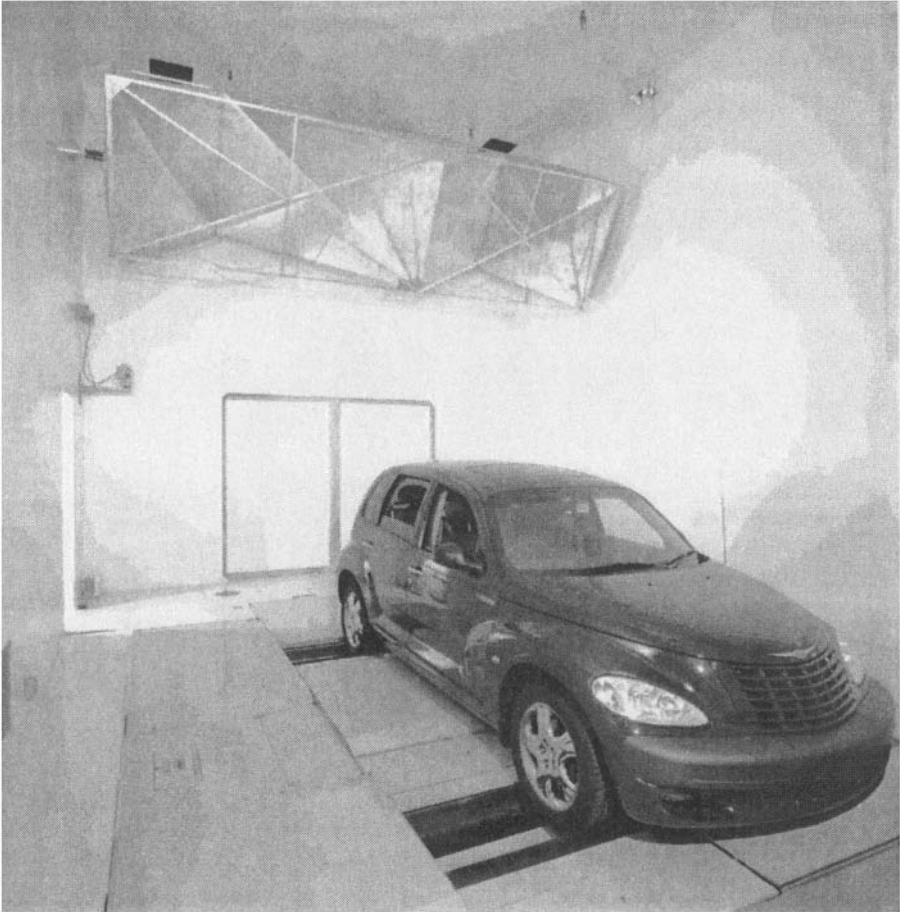
Figure 6.29 A Vehicle in a State of the Art Shielded Room Courtesy ETS-Lindgren, used with permission
