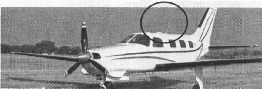
Figure 4.8. Ground "Plane" Antenna or "Grounded Plane Antenna"
