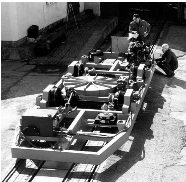
Figure 3.3 Parry People Mover chassis. The enclosed flywheel can be clearly seen in the middle of the vehicle (Photograph kindly supplied by Parry People Movers Ltd.)
