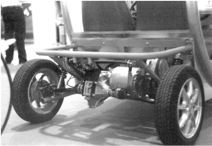
Figure 8.7 Example of type (a) of Figure 8.6 on an experimental electric vehicle by MES-DEA of Switzerland. The mounting of the motor is transverse, so there is no drive shaft
