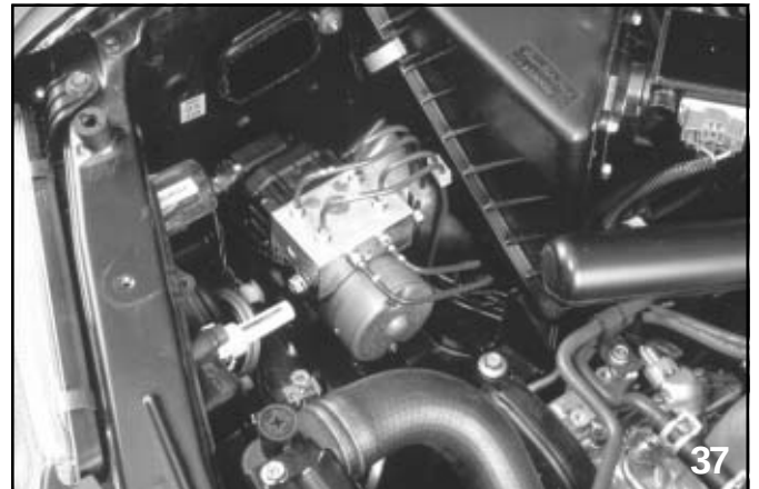
Hydraulic control unit
