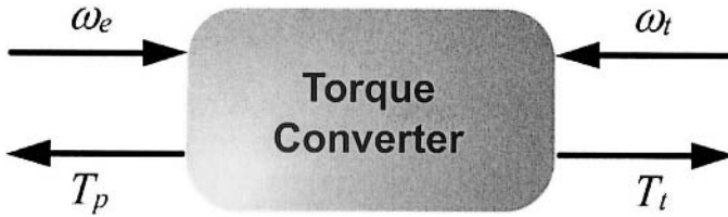
Figure 4-10. Schematic of torque converter model
