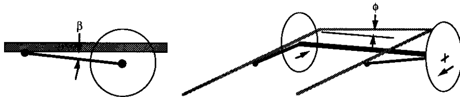
Fig. 6.16 Roll steer with a solid axle.
