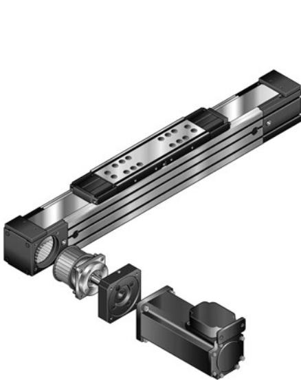
Fig. 4.14 Linear unit from Bosch Rexroth Group [7]. Depending on the application different variants are available: Assembled length; Custom servo, three-phase or stepping motor; Choice of planetary gearbox integrated in the timing pulley; Position detection; Control system
