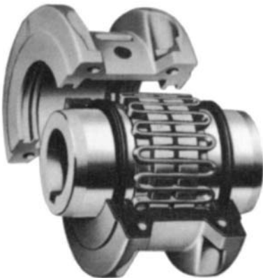
FIGURE 16.12 Metallic grid coupling with cover removed to show grid detail. (Falk Corp.)
