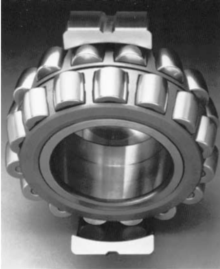
FIGURE 18.5 A spherical roller bearing with two rows of rollers running on a common sphered raceway. These bearings are self-aligning to permit misalignment resulting from either mounting or shaft deflection under load. ( SKF Industries, Inc. )
