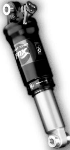
Figure 10.1 Fox Float RP23 used on the Marin Mount Vision. (Reprinted with permission of Fox Racing Shox.)
