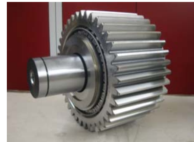
Fig. 11 Flexpin made by GDC GmbH
