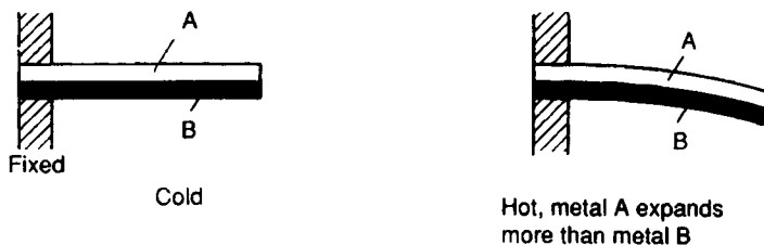
Figure 1.21 Bimetallic strip
