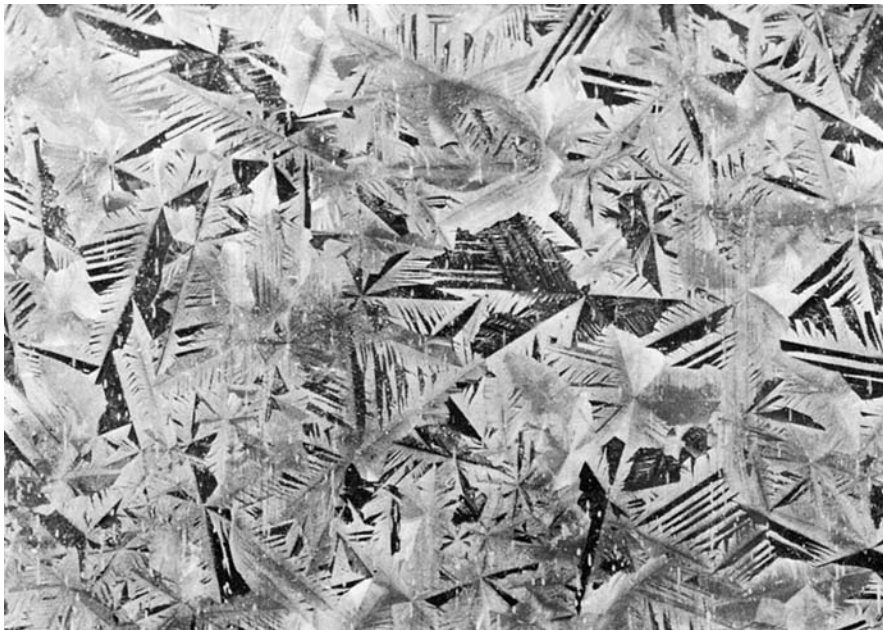
19.11. Spangles on the surface of a steel sheet that was hot-dip galvanized. From Making, Shaping and Treating of Steel , 9th ed. (United States Steel Corporation, 1971), p. 1032.
