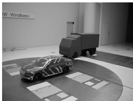
Fig. 2 Wind tunnel configuration in the case of overtaking process
