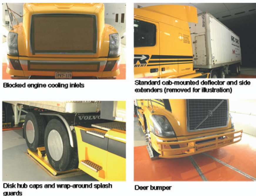
Fig. 3 Common components whose drag effects were measured
