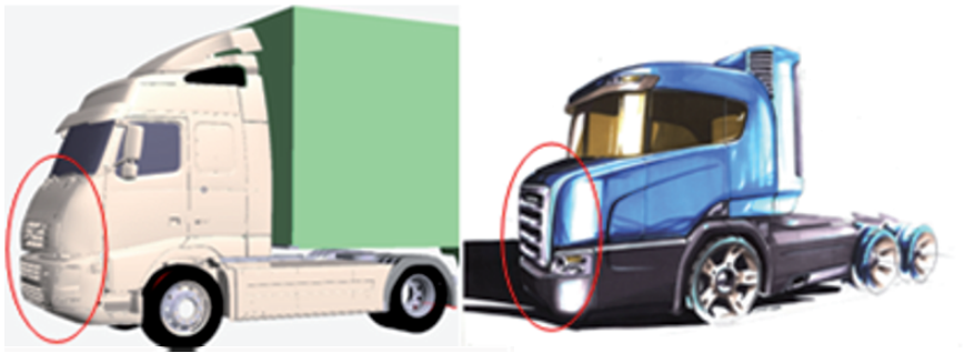
Fig. 6 Examples of “Crash nose” or “Soft nose”. Front face of the truck below the windshield extended approximately 300 mm forward.
