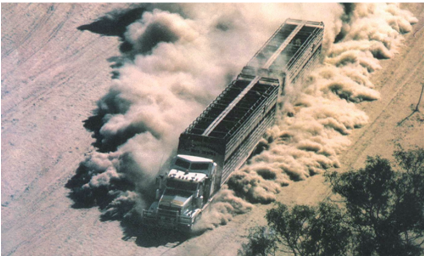
Fig. 10 Dust flow visualization from a cattle road train
