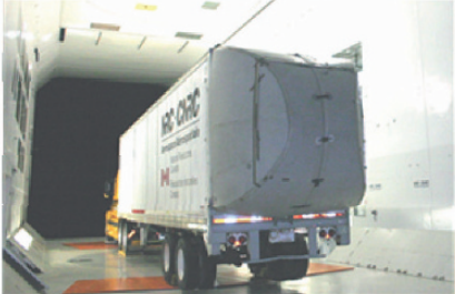
Aerovolution inflatable boattail
