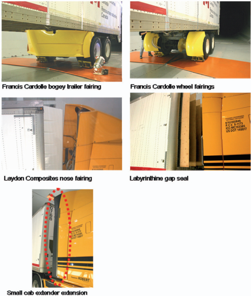
Fig. 5 New add-on components
