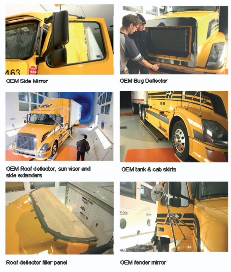
Fig. 2 Common components whose drag effects were measured
