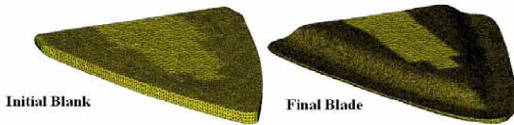
Figure 4: Microforming of surgical blades (Blank thickness = 0.1 mm; Final blade thickness = 0.01 mm) /7/.
