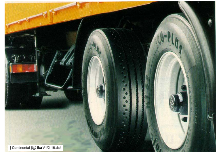
Fig. 2-16: Rolling resistance-minimized truck tire (Continental)
