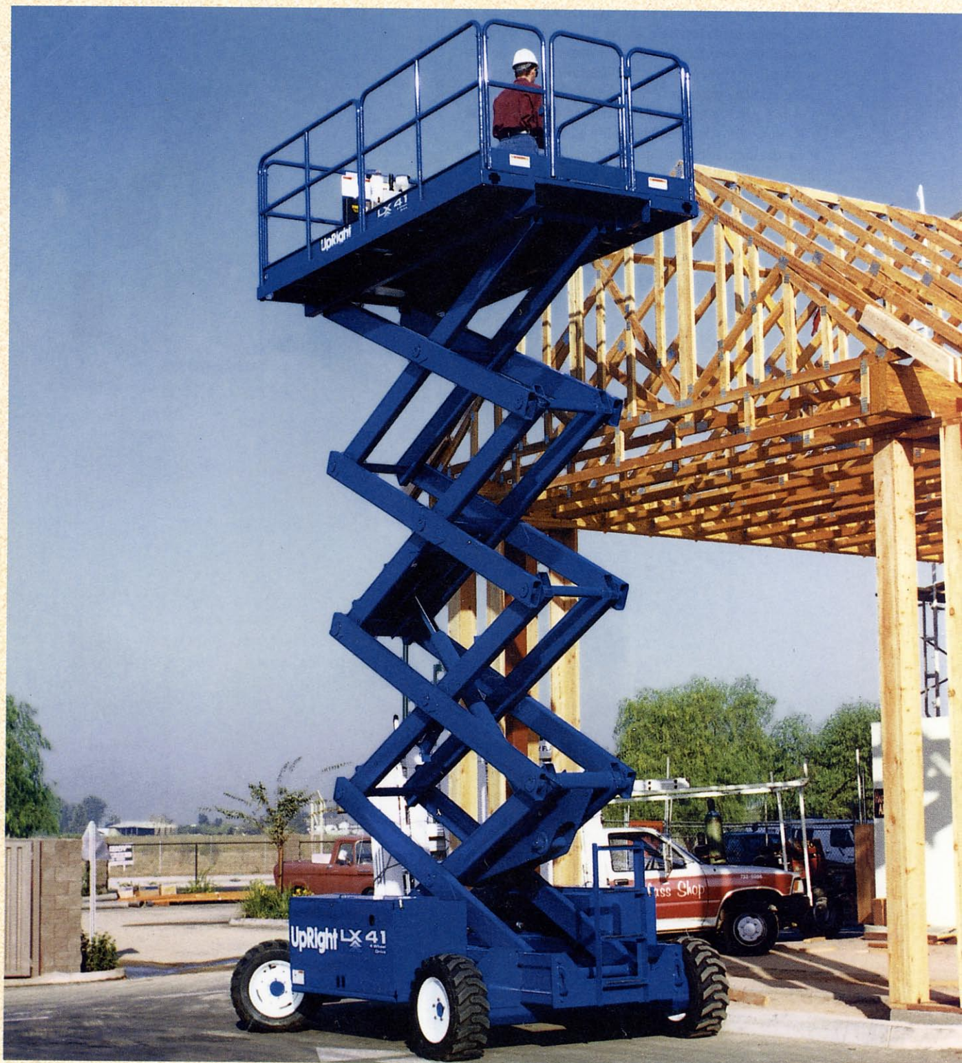
The analysis of multi-link structures which change configuration is generally best handled by a virtual-work approach. This construction platform is a typical example.
