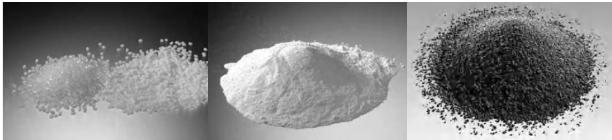
Fig. 2.23. Composites developed and commercialized by Rubitherm Technologies GmbH. From left to right: compound PK, powder PX, and granulate GR (pictures: Rubitherm Technologies GmbH).
