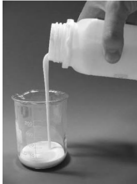
Fig. 9.43. Slurry based on microencapsulated paraffin (picture: FhG-ISE).
