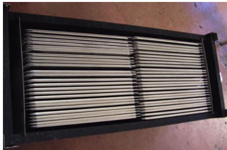
Fig. 9.31. Design of the storage currently developed by Rubitherm Technologies GmbH (picture: Rubitherm Technologies GmbH)
