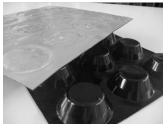
Fig. 2.28. Macroencapsulation in capsule stripes as produced by PCP and Dörken for inorganic PCM (picture: ZAE Bayern).
