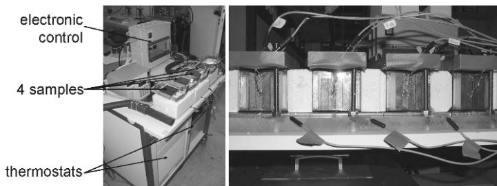
Fig. 3.31. Experimental setup for automatic heating and cooling of four samples and recording of the temperature over time (pictures: ZAE Bayern)
