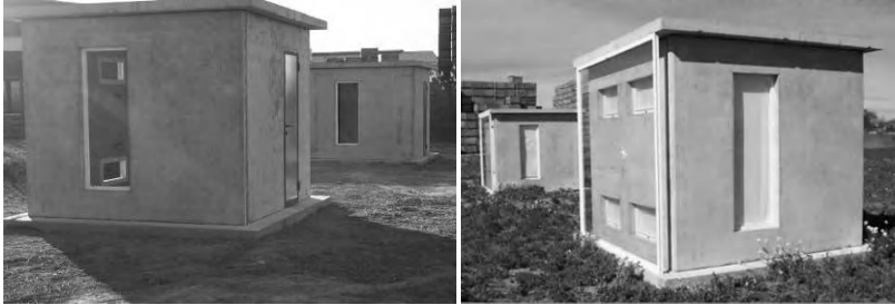
Fig. 9.13. Left: test buildings with walls from regular concrete and from concrete where microencapsulated PCM was added. Right: test buildings with additional trombe wall (pictures: University of Lleida).
