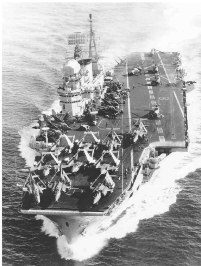
ABOVE: Eagle at speed in 1970, clearly showing her fully-angled flight deck.
