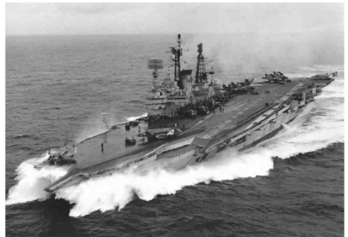
ABOVE: Ark Royal at full speed, in 1977, showing her appearance after her modernisation, with an 8½ degree angled flight deck, a forward projection to the steam catapult, and two Type 965 radars mounted atop an enlarged island superstructure.
