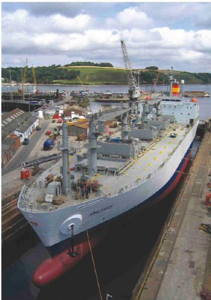
ABOVE: The geared general cargo ship Amazonas (1988/12,348gt) 'flooding up' in No.2 dock following a routine ten-day docking period.
