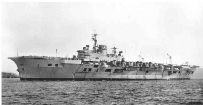
ABOVE: An early view of Eagle showing her appearance as completed, with a full battery of 4.5-inch guns visible.
