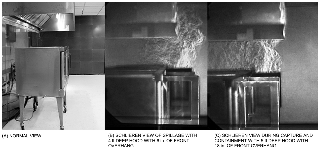
Fig. 8 Three Ovens under Wall-Mounted Canopy Hood at Exhaust Rate of 3400 cfm (Swierczyna et al. 2006)
