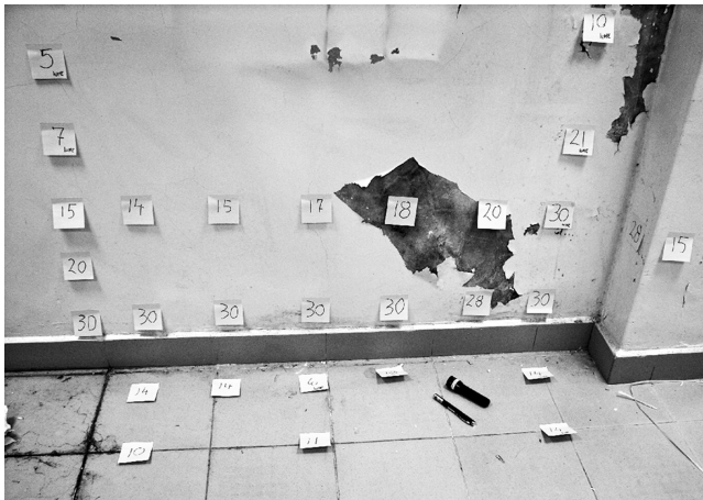
Fig. 8 Example of Documenting Both Values and Pattern of Moisture
