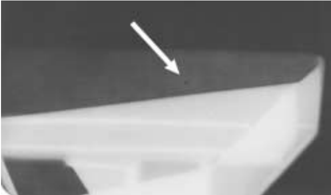
FIGURE 5. Gas discontinuities in 6.4 mm (0.25 in.) thick castings: (a) gas voids in steel; (b) round gas porosity in aluminum. 28
