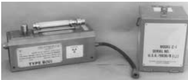
FIGURE 14. Exposure device with source exchanger: (a) exchanger (left) closed, exposure device fitted with short exchange tube; (b) exchanger open and attached, ready for source transfer to exchanger (note source pigtail in storage position, on the left).
