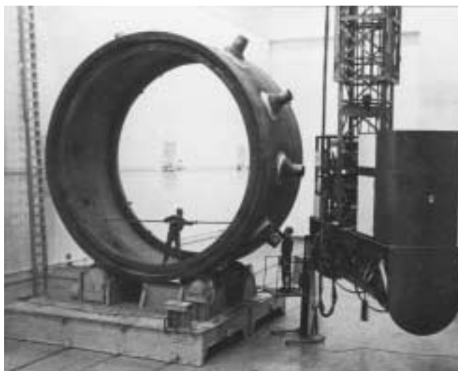
FIGURE 18. Placing film and aligning 13 MeV linear accelerator beam for examination of boiling water reactor nozzle weld. 20
