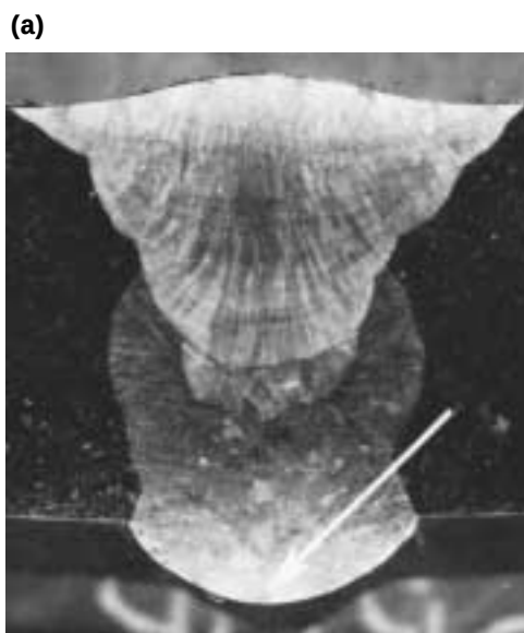
FIGURE 30. Drop-through: (a) photomacrograph at 4 \times ; (b) radiograph at 1 \times . 29
