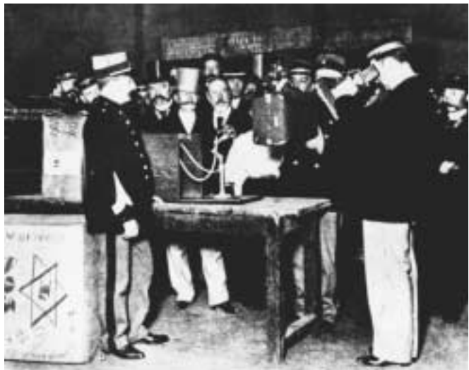
FIGURE 13. Radioscopic system for detection of contraband (circa 1910).
