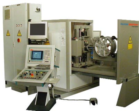
FIGURE 16. Radioscopy systems for automotive wheel inspection.
