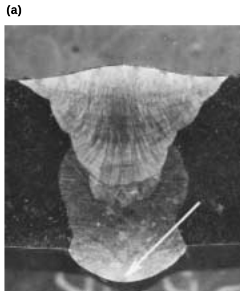
FIGURE 31. Excessive penetration: (a) photomacrograph at 4.5×; (b) radiographic image at 1.2×.
