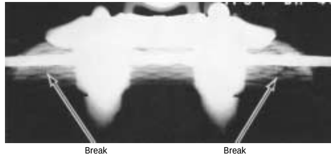
FIGURE 36. Radiograph showing multiple breaks under suspension clamp in field X-ray. 36
