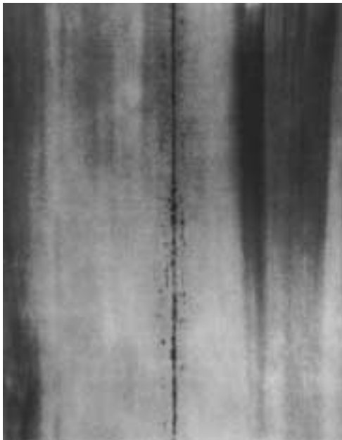
FIGURE 18. Streaking caused by inadequately cleaned film hangers.
