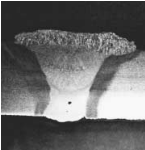
FIGURE 25. Hollow bead: (a) photomacrograph; (b) radiographic image.
