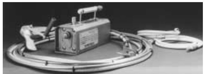
FIGURE 11. Exposure device with crankout and guide tube.
