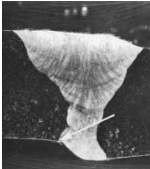
FIGURE 34. High low defect, also called mismatch : (a) photomacrograph at 4.4×; (b) radiographic image at 1.1×.
