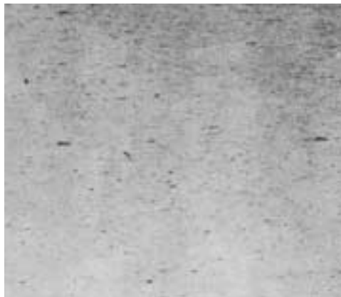
FIGURE 21. Surface deposits caused by contaminated wash water in automatic processor.
