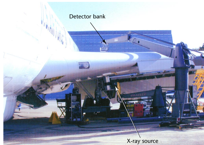
FIGURE 14. Setup for inspection of wing structure.
