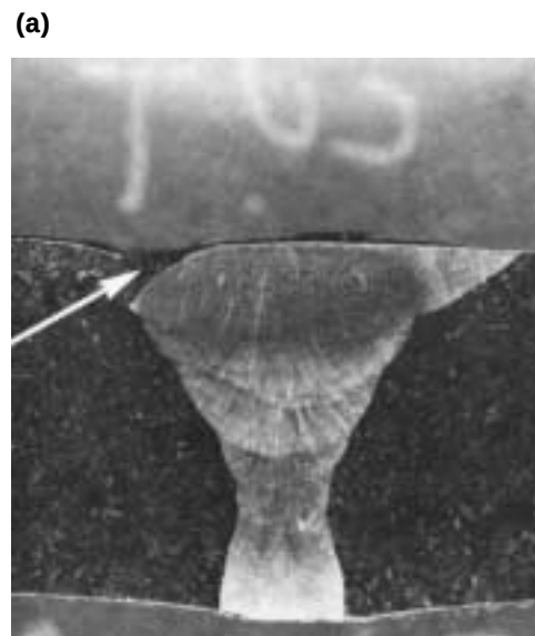
FIGURE 30. Undercut on outside diameter: (a) photomacrograph at 4.6×; (b) radiographic image at 1×.
