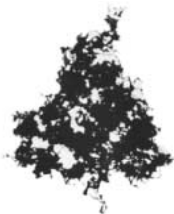
FIGURE 7. Electron micrograph of developed silver bromide grain.
