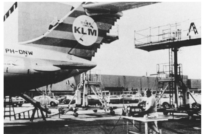
FIGURE 8. Position of X-ray source to expose maximum area of structure being radiographed.
