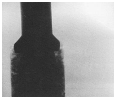
FIGURE 7. Medium magnification view of electrode seal in resistor spark plug.
