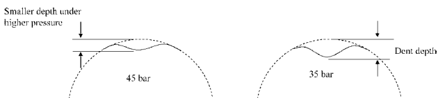
Figure 6.13 Re-rounding effects on dents
