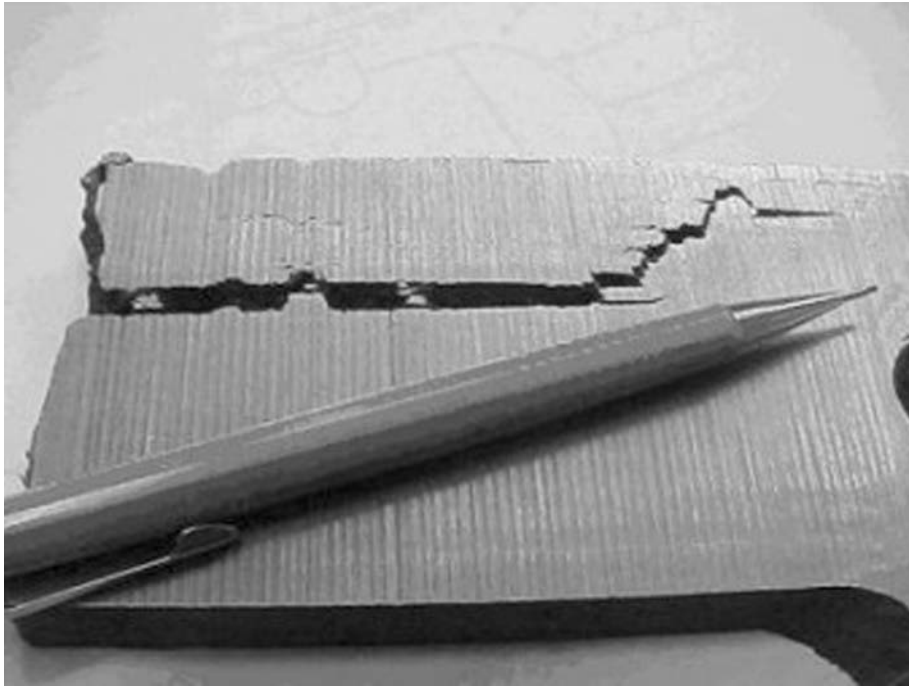
Fig. 5-22—Cross-section of plate showing HIC damage in the shell of a trim cooler which had been cooling vapors off a HHPS vessel in a hydroprocessing unit.
