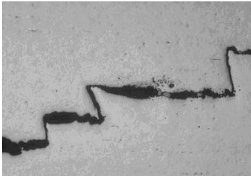
Fig. 5-24—High magnification photomicrograph showing stepwise cracking nature of HIC damage.
