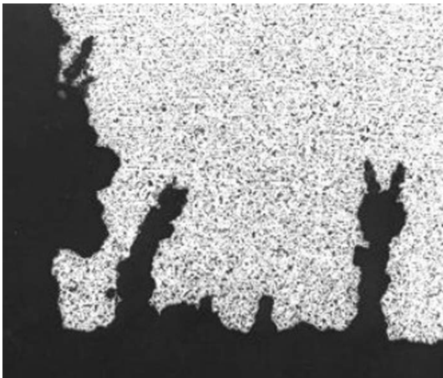
Fig. 4-84—Photomicrograph showing the crack morphology that is rounded with multiple lobes, and may branch to form "rabbit ears." (Mag. 25×, etched)
