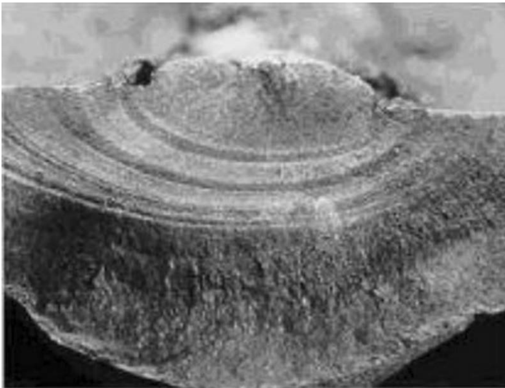
Fig. 4-30—Fatigue fracture surface of a carbon steel pipe.
