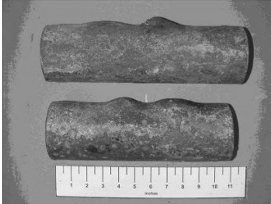
Fig. 4-9—Short term overheating of a fired heater tube.
