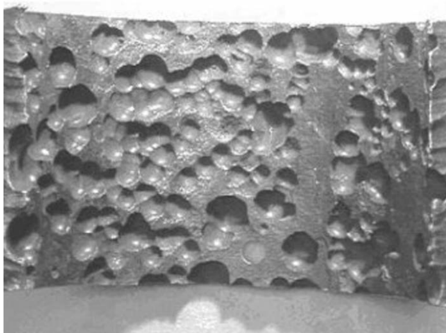
Fig. 4-70—Metal dusting of a 304H stainless steel pipe.
