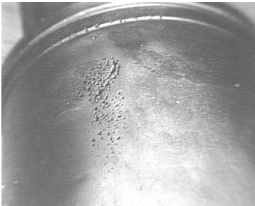
Fig. 4-28—Cavitation pitting on the water side of a cast iron cylinder liner in a large engine.
