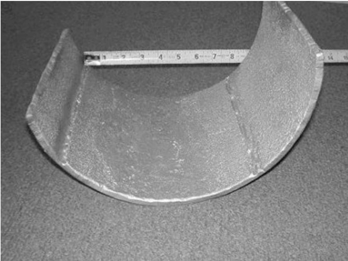
Fig. 5-10—Grooving corrosion in the carbon steel vapor line from an alkaline water wash drum in a sulfuric acid alkylation unit.
