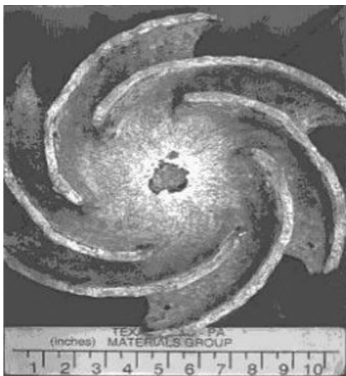
Fig. 4-24—Cast iron impeller in untreated cooling water after four years of service.
