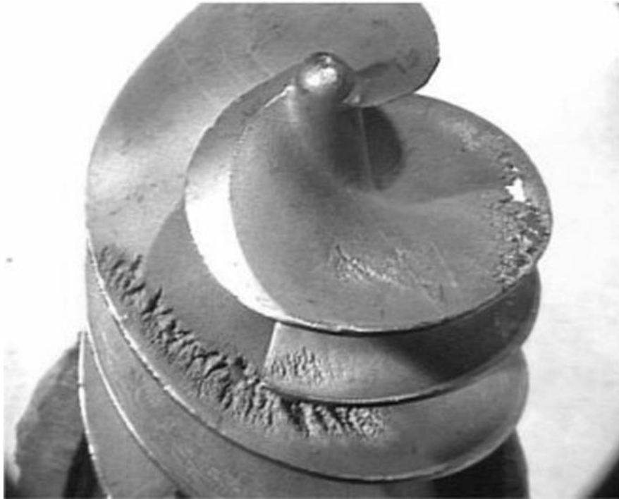
Fig. 4-27—Cavitation pitting on the low-pressure side of a stainless steel pump impeller.
