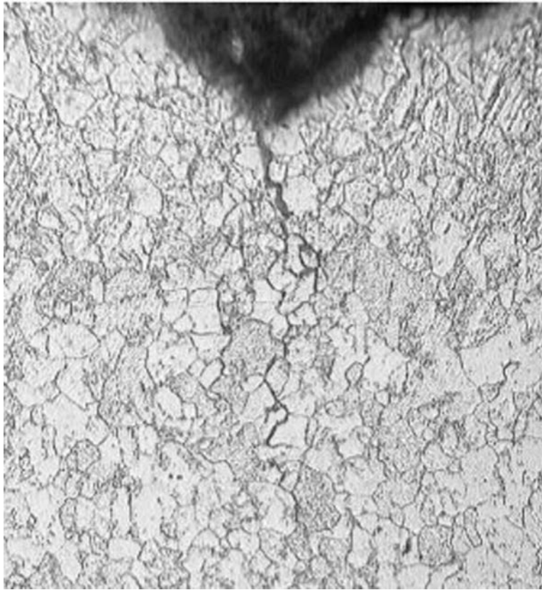
Fig. 4-87—Photomicrograph of a crack in the tube shown in Figure 4-86.
