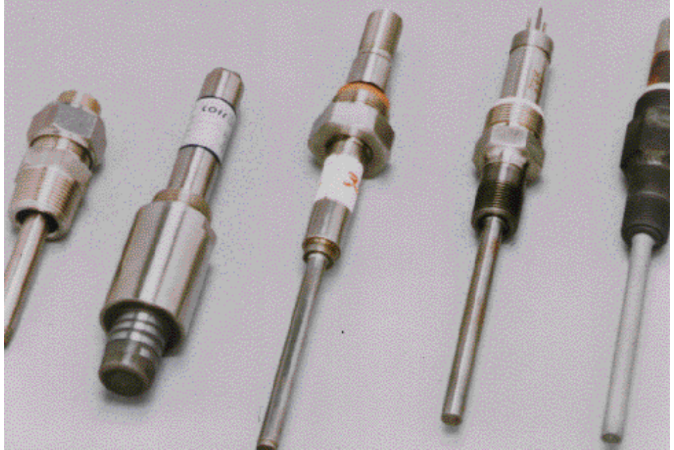
Figure 17a: Typical ER Probe Designs
