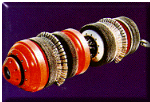
Figure 7.8 MFL In-line Inspection Tool
