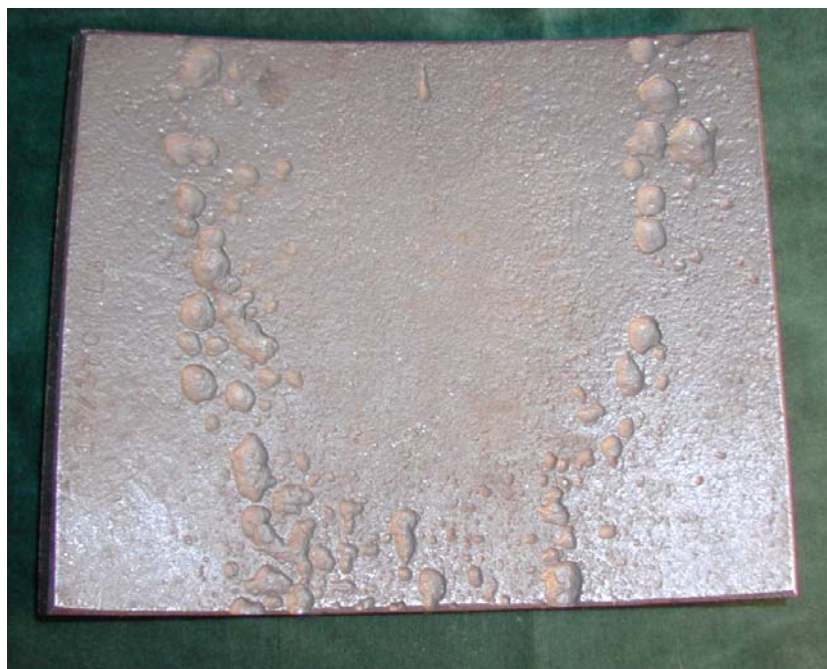
Figure 10.1 Internal Corrosion Cluster in Crude Oil Production Line (with High CO 2 )
