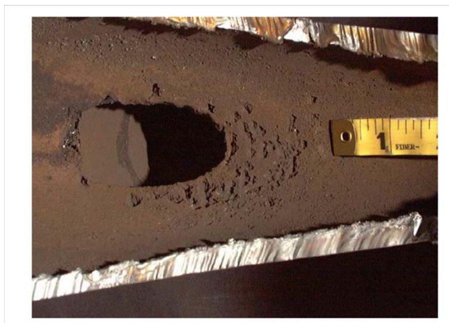
Figure 2.15 Example of a Local Impingement Attack in High-Velocity Flow
