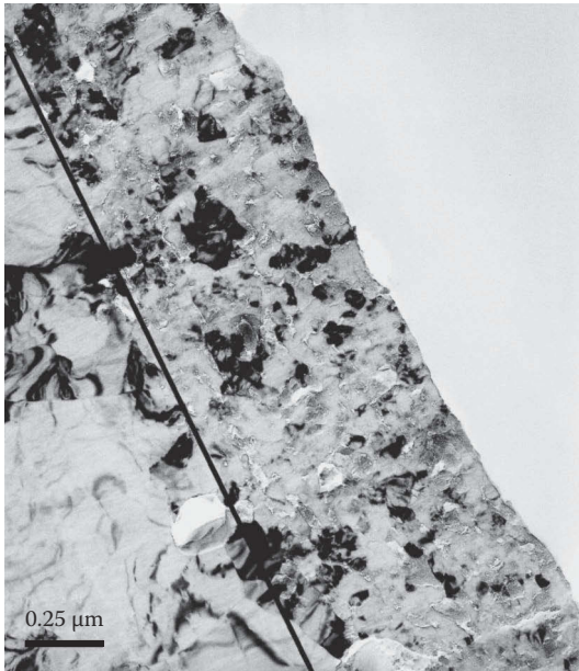
FIGURE 12.8 Deformed surface layer on rolled aluminum. The deformed layer to the right of the black line is formed during rolling and is characterized by nanosized grains, rolled in aluminum oxide fragments and small intermetallic particles. The presence of such layers makes coated aluminum highly susceptible to filiform corrosion, particularly if the alloy has been heat treated to temperatures of >350^{\circ}\text{C} before coating.
