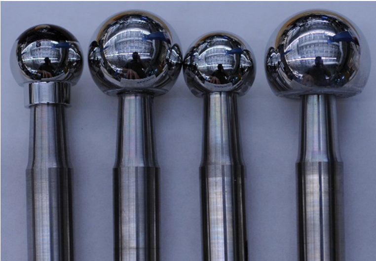
FIG. 2 The femoral heads used in this test. From left to right (all dimensions are in millimeters diameter + offset): 28 + 12 , 36 + 12 , 28 + 8.5 , and 40 + 8.5 .
