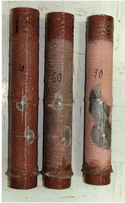
Figure 6-1. Cathodic disbondment test (ASTM G-8) shows growth of the disbondment area from 30 to 60 to 90 days.
