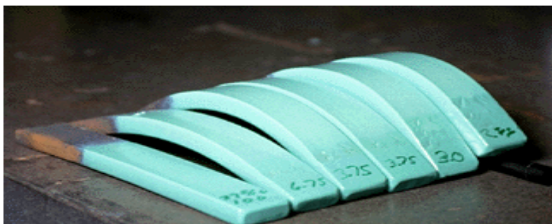
Figure 6-4. Facility and the specimens for testing of flexibility of coatings.
