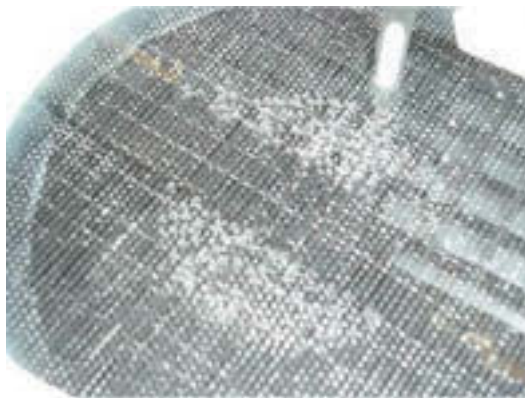
Figure 6-7. Testing for non-shielding properties of mesh-backed tape show hydrogen evolution.
