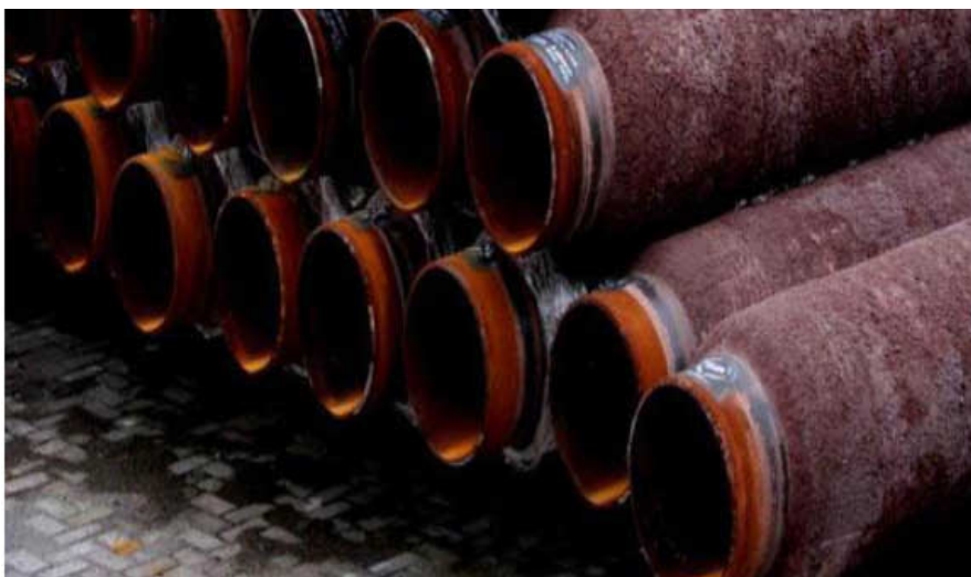
Figure 3-2. Coal tar enamel coated steel pipes in storage (concrete coated).
