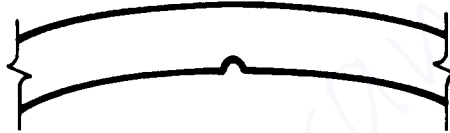
If hole is for positioning or indexing, try a small notch instead
