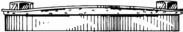
Figure 2.3 Illustration of flange bending or bowing.
