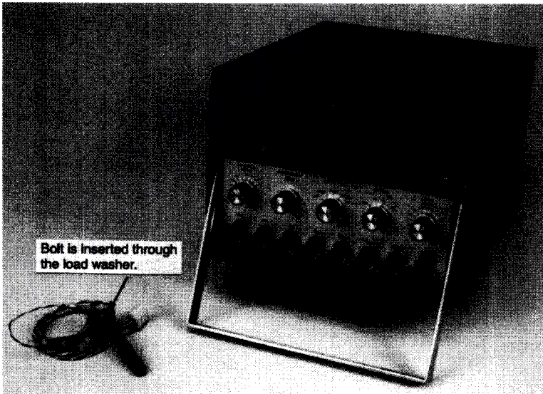
Figure 7.16 Load washer, bolt, and strain indicator.
