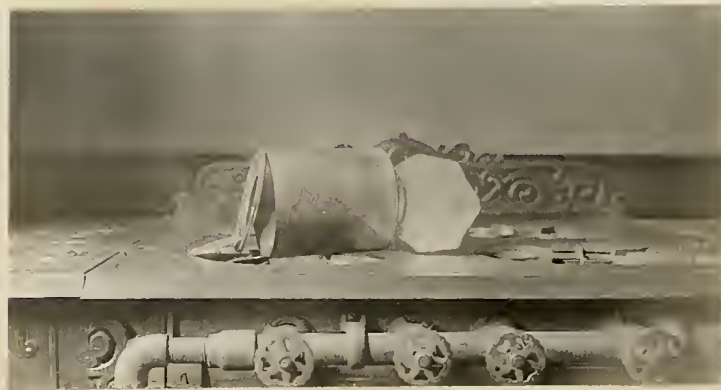
Remove the end of a tin can by melting the solder.
