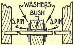
FIG 3 SECTION OF FRONT OR REAR WHEEL
