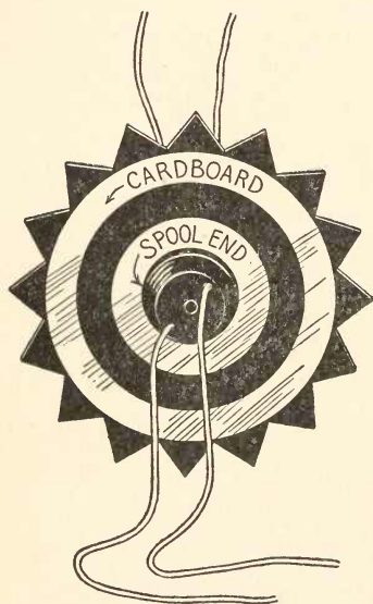
FIG. 111. — Detail of Buzz-Saw Whirligig shown in Fig. 108.
