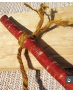
Fig. A: Gather wood, string, and a knife. Fig. B: Whittle a spindle with semi-pointy ends. Fig. C: Notch the handhold to seat the spindle. Fig. D: Tie a thick string to the bow ends. Fig. E: Drilling stance (rightly): left foot on the
