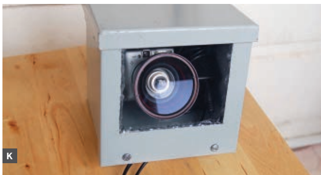
washer, screw, and bolt. Fig. J: Cut a notch at the front of the box floor for the USB cable. Fig. K: Adjust the set-screw to ensure that the power is on, then plug in the AC adapter and stuff it and the camera inside the enclosure.
