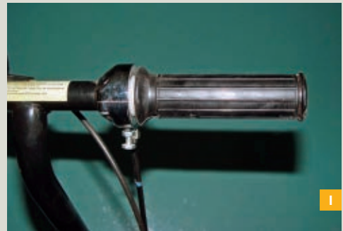
Fig. D: Rear axle and brake moved back on the swing arm to accommodate a larger rear wheel. Fig. E: Right-angle gearbox mounted to a custom tapped plate that's screwed to the original motor mount. Fig. F: Aligning the sprockets. Fig. G: Wooden kickstand extension. Fig. H: Gearbox shaft milled into a triangular shape, for a stronger hold from the drill chuck. Fig. I: Handlebar twist-grip for throttle cable. Fig. J: Throttle mechanism, cable side.
