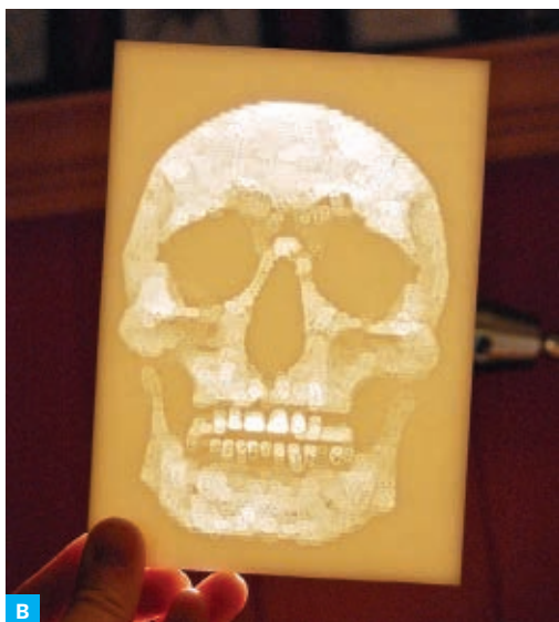
Fig A: My micRo CNC robot, built from a kit. It was easy. Fig. B: The bot milled this plastic to different depths, using a simple CAM program.
