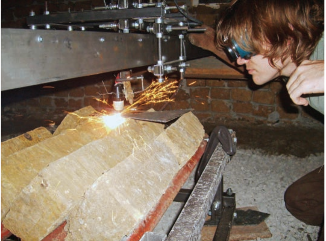
IN THE THICK OF IT: (Opposite) Lawrence Kincheloe and Marcin Jakubowski pose inside the RepTab cutting table. (This page) Kincheloe practices cutting with the plasma cutter tip on the RepTab.
