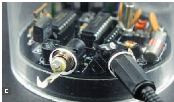
Fig. D: The mini Geiger-Müller tube wrapped with copper foil. Fig. E: Holes drilled in the main tube for power and data connections.
