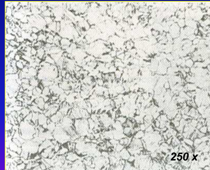
Air-cooled from \alpha+\beta phase field, showing primary \alpha grains in a matrix of transformed \beta (acicular)
