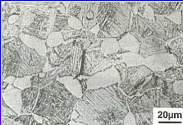
Crack initiation at lamellar region in bi-modal microstructure
