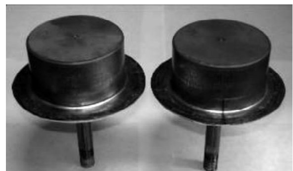
Fig. 13. Cylindrical specimens produced by SPF out of sheet blanks of nanostructured VT6 alloy (average grain size – 0.2\ \mu\text{m} ) at 600^{\circ}\text{C} (right) and 650^{\circ}\text{C} (left) [44].
