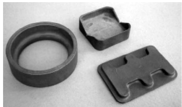
Fig. 11d. Rings, flanges produced by precise die forging in superplastic conditions.
