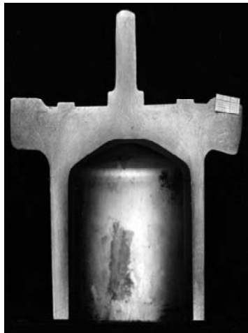
Fig. 9. Longitudinal section from cylindrical billet. X1.2.
