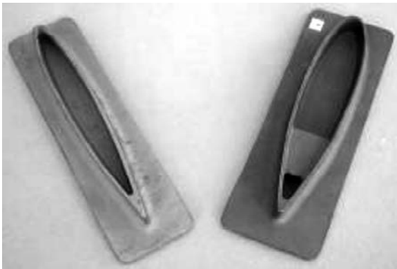
Fig. 11e. Frames produced by precise die forging in superplastic conditions.
