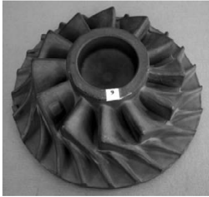
Fig. 11a. Disc with blades produced by die forging in superplastic conditions.
