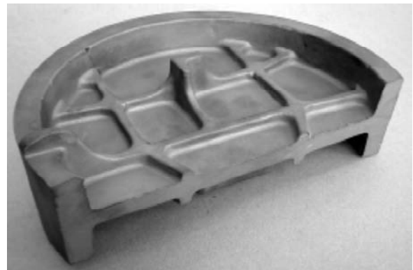
Fig. 11f. Complex profile "frame" type article out of titanium alloy.
