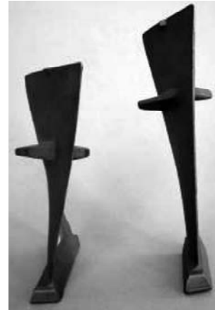
Fig. 11b. Blades of gas turbine engine compressor produced for one operation step.
