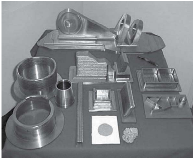
8.27 Examples of Lasform shapes (courtesy AeroMet Corp.). A further example of an ALM component is shown in Fig. 8.28.
