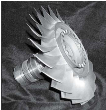
8.35 ALM repair of gas turbine components.
