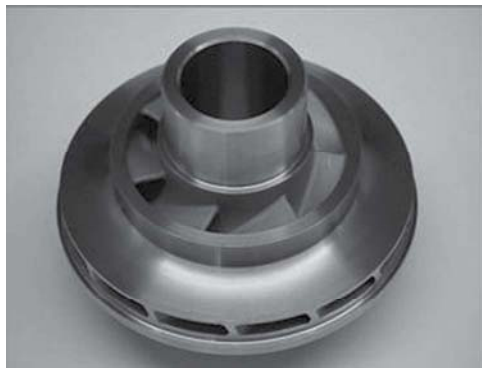
8.23 Selectively net shape ELI Ti-6Al-4V impeller for a turbo-pump of a rocket engine. Fabricated using the prealloyed metal method (courtesy Synertech PM/P&W Rocketdyne).
