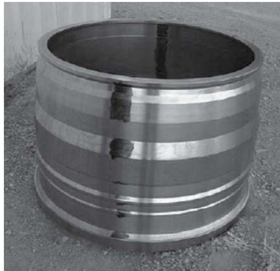
8.34 Fan case produced by adding features by ALM to a forged preform.
