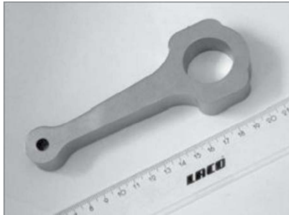
8.6 Auto connecting rod fabricated via the blended elemental approach using hydrogenated titanium powder (courtesy Orest Ivasishin, Ukrainian Academy of Sciences).
