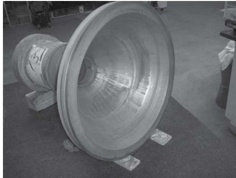
8.22 Near net shape Ti-6Al-4V engine component fabricated using the prealloyed metal mold method (courtesy Synertech PM).
