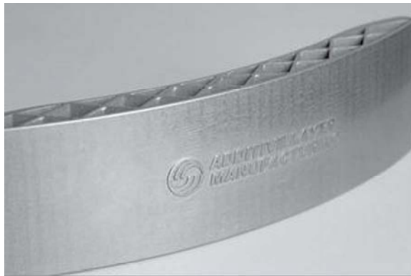
8.28 Additive layer manufacturing. Sandwich structure aerofoil demonstrator produced at the Centre for Additive Layer Manufacturing (CALM) using an electron beam chamber and powder feed.
