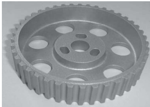
8.32 Automotive pulley prototype fabricated by ALM.
