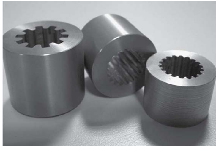
8.40 Titanium heat pipe connectors produced by cold spraying (courtesy of M. Jahedi, CSIRO).
