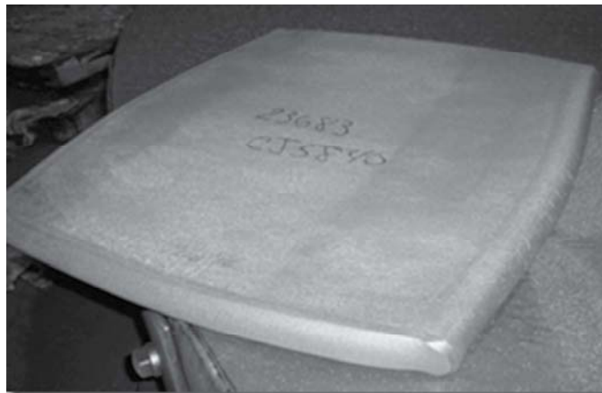
8.47 Cold press, sinter and hot rolled preform (weighing 95 kg (210 pounds)) for commanders hatch forging (Bradley Fighting Vehicle) (courtesy of ADMA Products).
