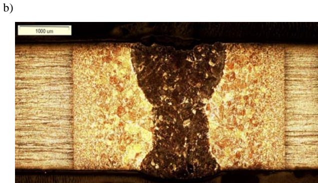
Fig. 4 Macrograph of the cross section of butt joints of titanium alloy Ti6Al4V sheets 2.0 mm thick laser welded with the Disk laser; a) joint no. Z2, b) joint no. Z3, Table 4
