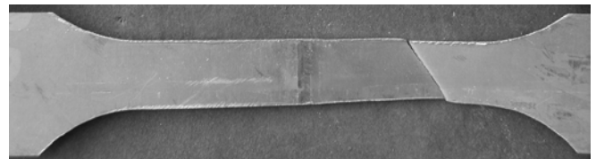
Fig. 10 A view of the titanium alloy Ti6Al4V butt joint Z3 after tensile test, Table 4
