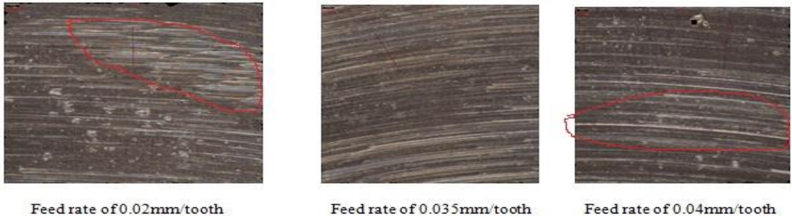
Figure 7.7 - Surface images of the test cut at different feeds.
