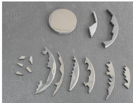
Figure 3.6 - PCD blanks and chips cut by W-EDM.
