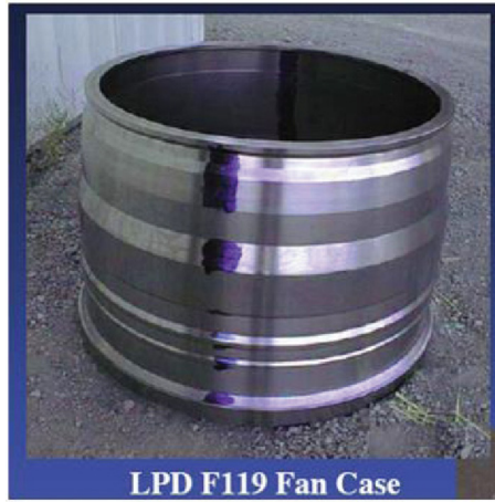
Figure 24.9 Fan case produced by adding features with AM (laser-aided directed energy deposition) to a forged perform. (Courtesy Jim Sears.)
