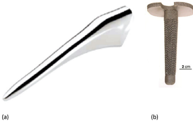
Figure 24.8 Medical implant application using; (a) DMLS technology. (Courtesy Jim Sears.) (b) EBM technology [26].
