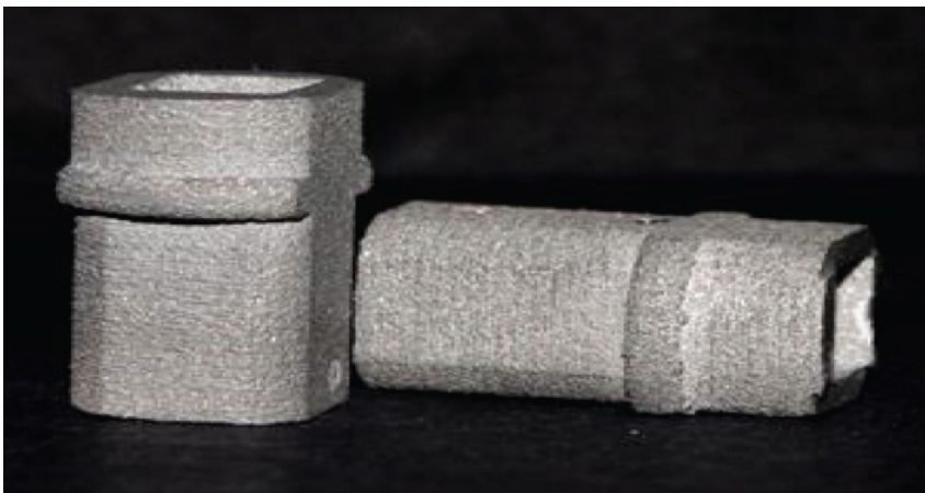
Figure 24.20 Automotive component produced from Metalysis powder after spheroidization of the powder [39].
