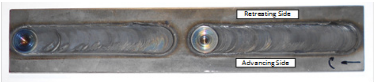
Figure 7. Ti-6Al-4V FSW workpiece (260mmx50mm) after FSW process, AS: advancing side of the tool, RS: retreating side of the tool.
