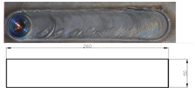
Figure 5. Macrograph of the stir zone surface and its dimensions in millimeters.
