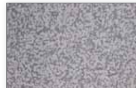
Alpha-beta alloy Ti6Al4V showing primary alpha grains and a fine alpha-beta matrix structure.
