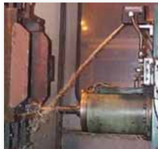
Inadequate coolant delivery
