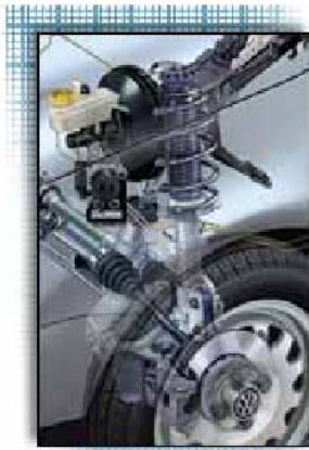
Figure 10. Volkswagen Lupo FSI with TIMETAL LCB suspension springs
