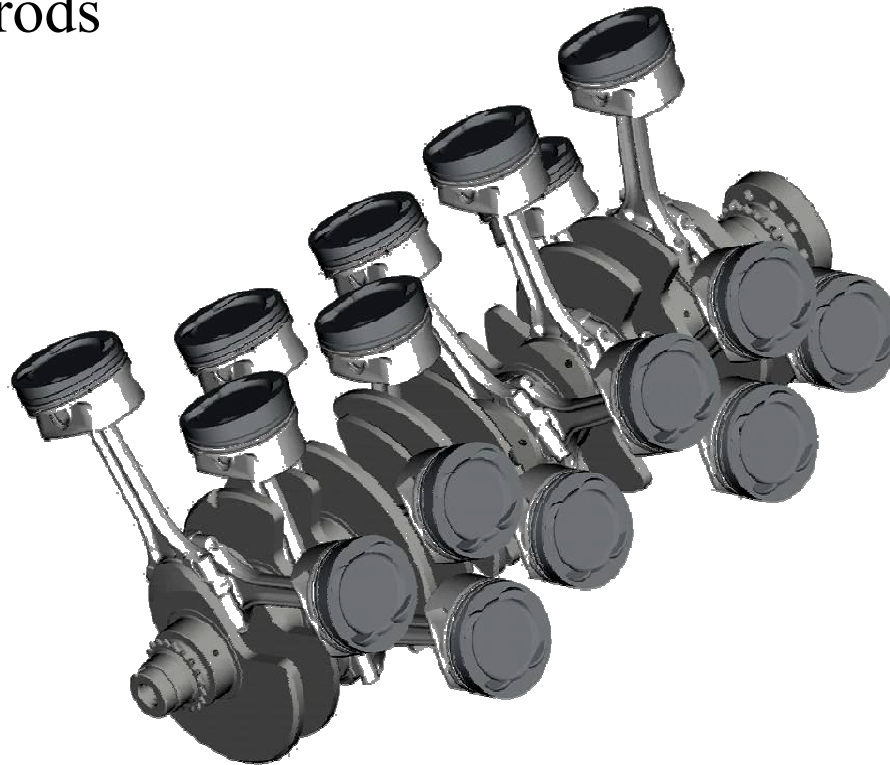
Figure 2. Ti-6Al-4V connecting rods in the Bugatti Veyron 16.4 8-liter W16, 4 turbo chargers, 2 liquid intercoolers, 1001 HP, 922 lb-ft
