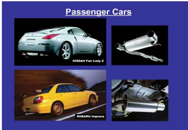
Figure 5: Application examples of titanium exhaust systems in Japanese passenger cars
