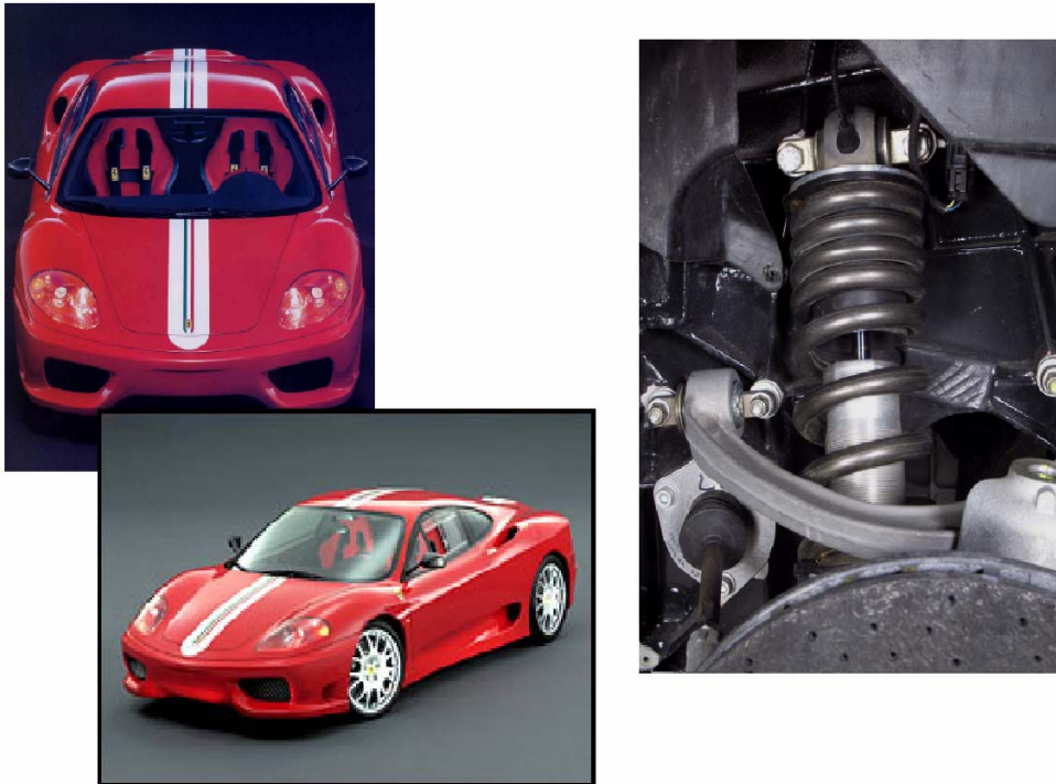
Figure 11. Ferrari Stradale 360 with LCB springs (courtesy of TIMET company) 3.6-liter V8, 425 HP
