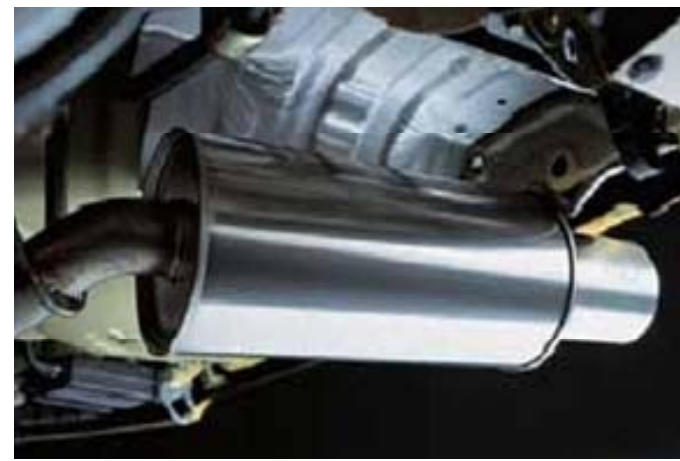
Figure 5. Application examples of titanium exhaust systems in Japanese passenger cars (courtesy of Toshihiko Saiki)
