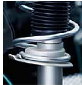
Figure 10. Volkswagen Lupo FSI with TIMETAL LCB suspension springs
